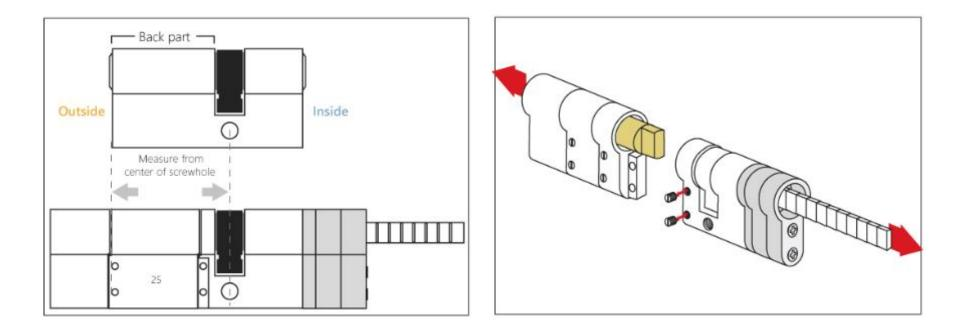
4. Unscrew the small screws on both sides of the cylinder and pull it apart.
