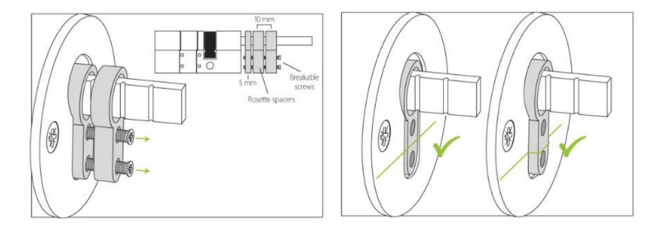
**IMPORTANT!** Avoid pulling the cylinder out of place. It is important that the spacer flushes or sticks out from the hole in the rosette plate.
