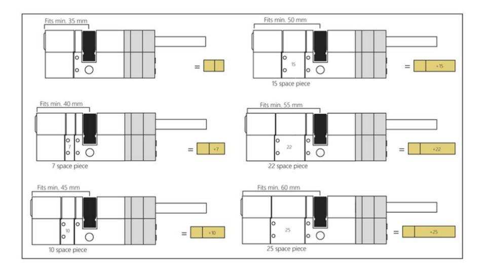
**Size guide** - When you adjust the size of the Danalock cylinder to the old cylinder you'll have to exchange the brass tube in the center with another that fits the spacer piece. Here are the different combinations.
